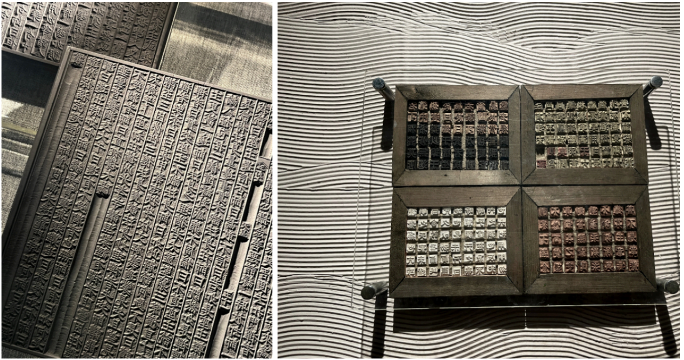
Fig. 5 Woodblock printing block and movable types for Hanzi. Photo by the author, China Block Printing Museum, Yangzhou, China.
